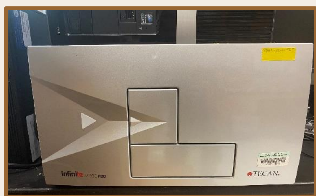
Figure 4: Spectrometer used to test phenolic and tannin absorbance.
